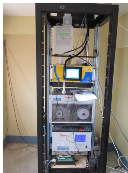
Fig. 2. Upper picture: landscape of Kathmandu valley from the Suskat Observatory at the Ev-K2-CNR Representative Office in Pakanajol. On the right: Internal view of the Suskat Station at Pakanajol: condensation particle counter, OPC, MAAP and O 3 analyser.
