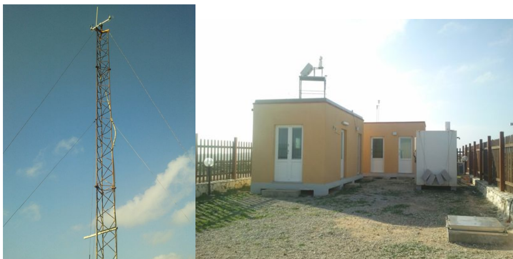
Figure 3. Left: Weather tower in the experimental field of the “R. Sarao” station. Right: transportable modules housing laboratories for aerosol sampling, ozone analyzer, the PSAP, the Cimel, and a clean room for the treatment of aerosol samples for chemical analysis.
