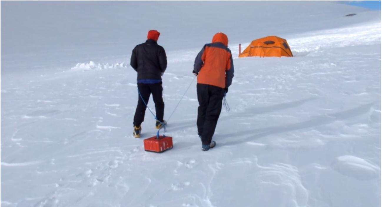
Fig 20. Performing radar surveys at the Gasherbrum Glacier surface.
