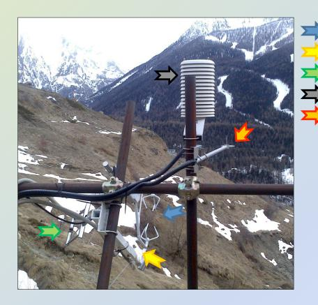
Tridimensional sonic anemometer Infrared gas analyser (Licor) Kripton hygrometer Thermo-hygrometer Net radiometer Soil heat plates  $(x^2) - 6$  cm (thermocouples) TDR soilmoisture probes  $(x_2) - 8$ , 20, 40 cm Soil thermometers (x4) - 2 e 8 cmSurface infrared thermometer CR3000datalogger Photovoltaic electrical supply Nearby ARPA meteorological station
