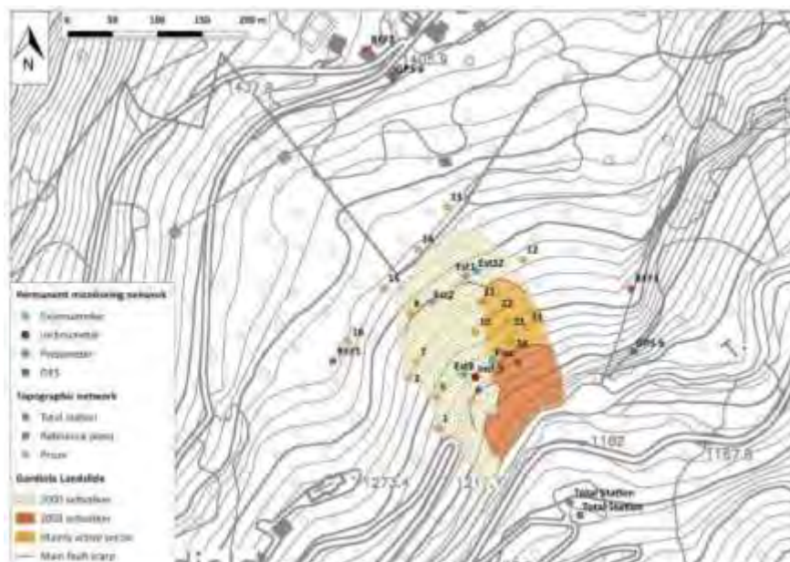
Figure 2.2 – Permanent monitoring network of Gardiola landslide represented in Qgis
