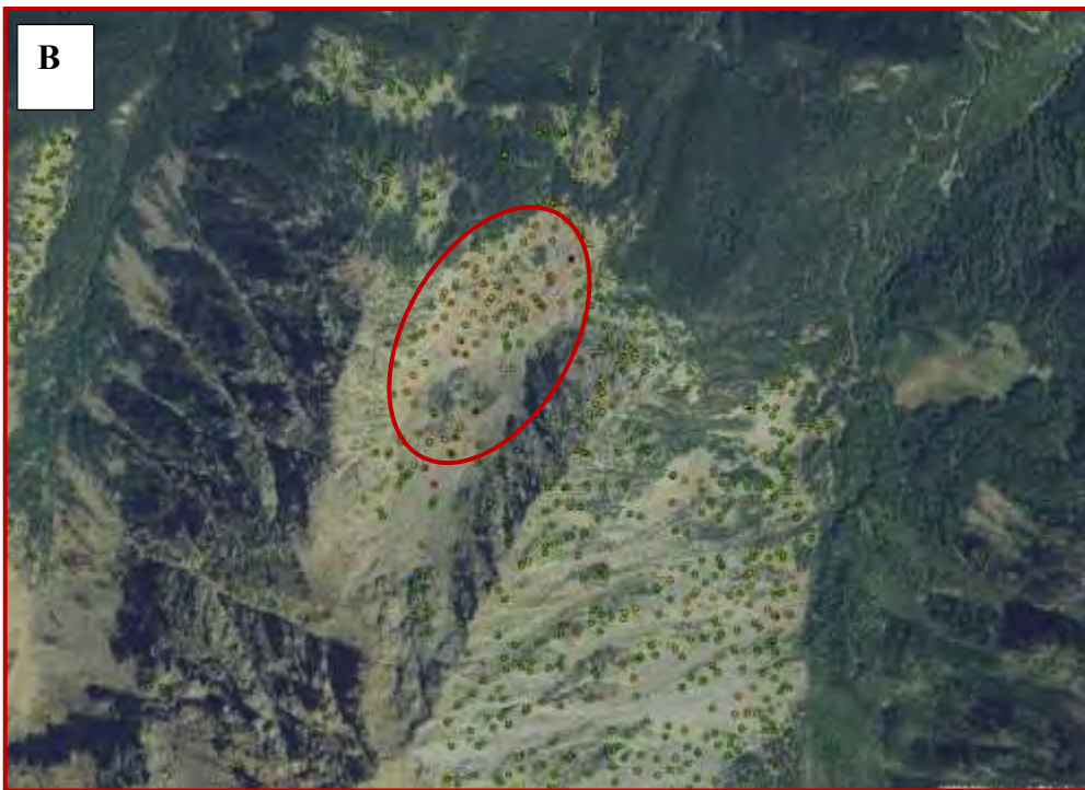
Figure 3.6 – La Clapey Gerbioz rock glacier; A) ground deformation distribution obtained with SBAS technique by G-POD service, for Envisat ASAR satellite composed by 39 images in ascending orbit, for the period 2004-2010; B) ground deformation distribution showed on “Portale Cartografico nazionale” obtained with PSInSAR technique for Envisat ASAR.
